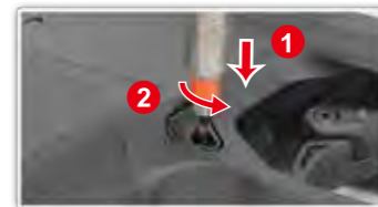
Push down the screw with flat head driver, then turn 90 degree counter clock-wise.
