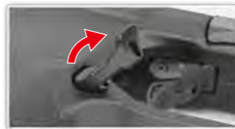
Push out the button from the other side of the pistol.
