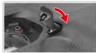
Switch to the other side of the pistol and install the button from the top.
